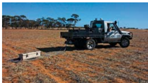
The EM38 (in box behind vehicle) can produce rapid, paddock-scale soil surveys of some soil properties.
