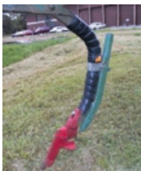
Pig's Tail wrapping on a John Shearer 620 shank. NSW trials showed potential residue handling benefits esp. with edge-on and spring coil tines (see www.weldalloy.com )
