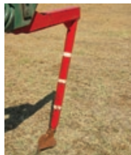
High clearance straight shanks with circular section promoted superior residue handling in SA trials
