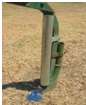
Trash guard shape should be optimised to minimise increases in soil throw
